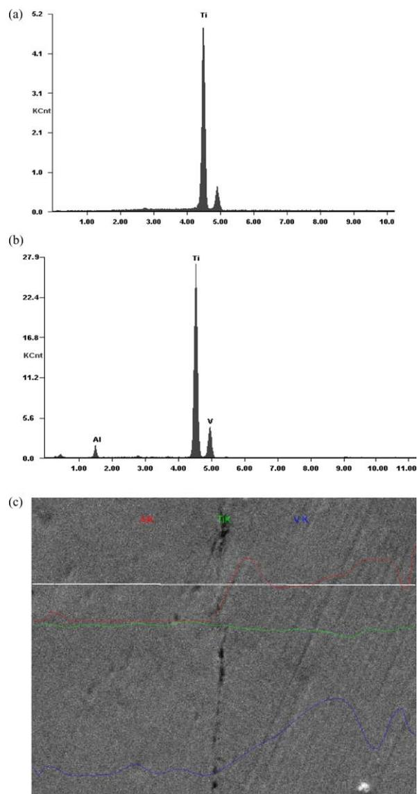
**Figure 3** X-ray EDS spectra of the brackets. (a) Orthos2 bracket base showing that the bracket is composed of Ti. Similar to the spectrum of Rematitan. (b) Orthos2 bracket wing showing the presence of Ti, Al and V. (c) X-ray line scan images of the elemental distribution of Ti, Al and V at the base-wing interface revealing increased Al and V concentration at the wing component. Note the interfacial porosity.
