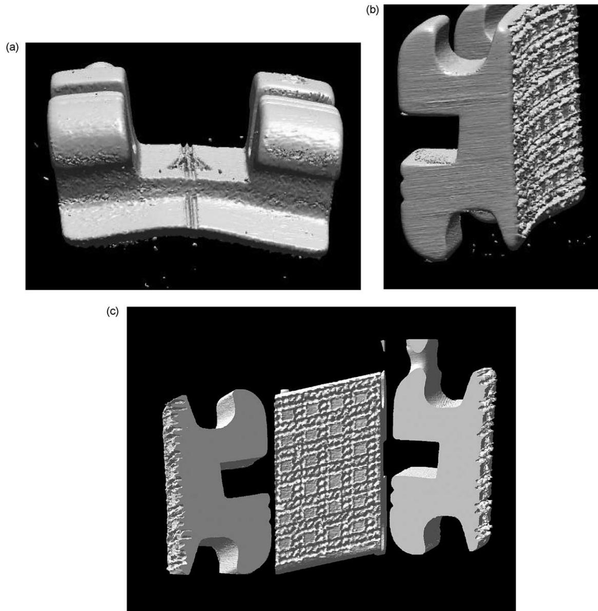
**Figure 2** 3D X-ray microtomographic image of a Rematitan bracket. (a) Detail of the outer base-wing region showing a smooth transitional zone. (b) View of the base mesh at an angle depicting the laser-etched base and the smooth base-wing transitional zone. (c) Face view of the base mesh demonstrating the non-welded base-mesh pattern and tomographic sections revealing a continuous base-wing interface.
