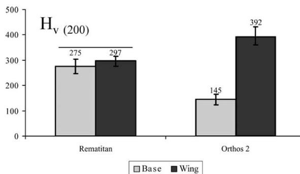
**Figure 4** Vickers microhardness ( $HV_{200}$ ) for the base and wing components of the two bracket types tested. Bar indicates values of no statistical difference ( $p > 0.05$ ).
