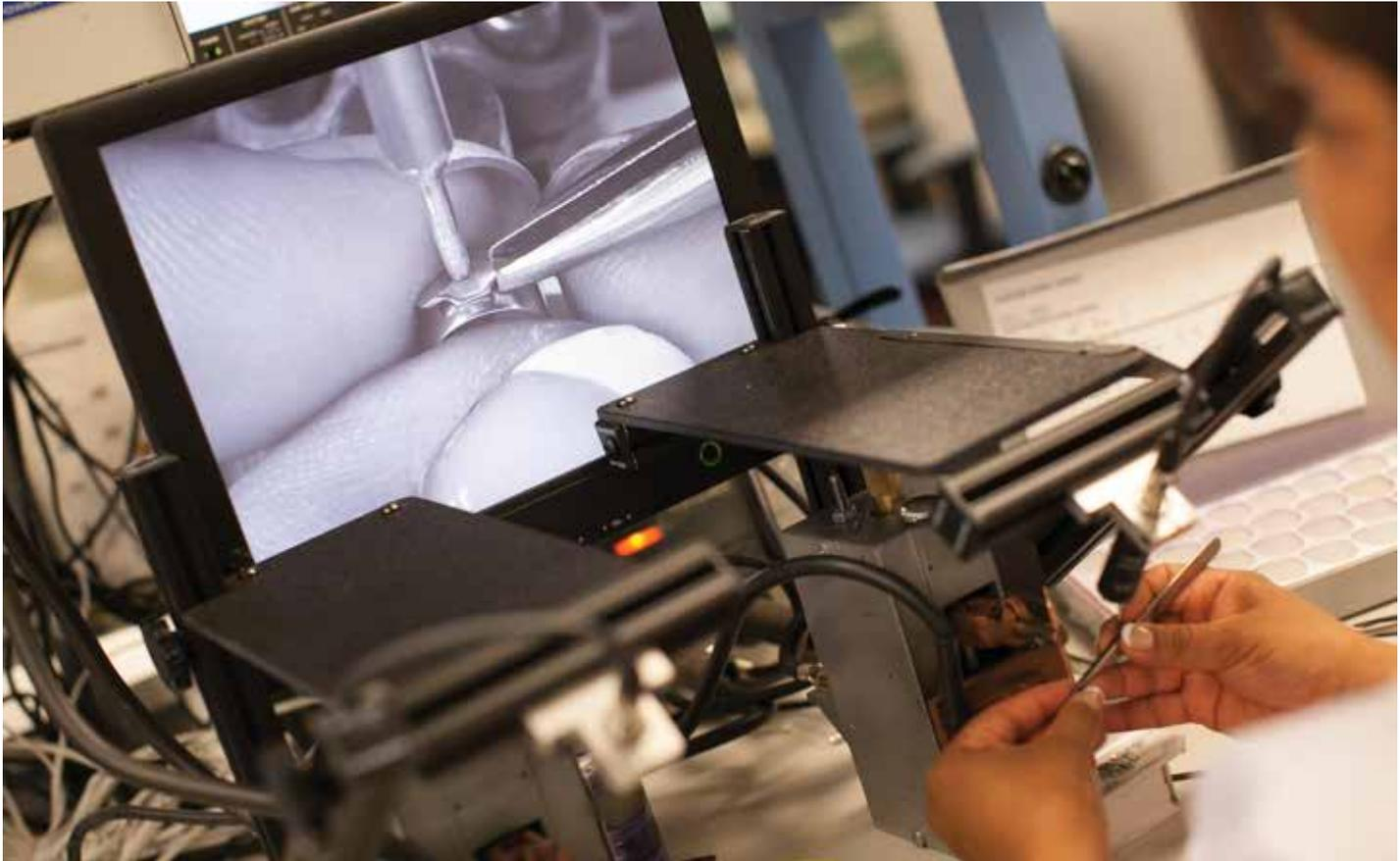
"Ormco" is an acronym for Orthodontic Research and Manufacturing COmpany. In this photograph, an Ormco technician tack welds a lingual cleat to a band during the manufacturing process
